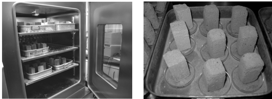
Fig. 2 – Chlorides resistance test: samples in the climatic chamber and deterioration of the samples
