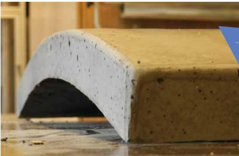
"Flexible mould" method: a way to manufacture curved concrete elements by deformation after casting; the image shows a demoulded, clearly curved, concrete element of 50 mm thickness. Credits: Roel Schipper, TU Delft
