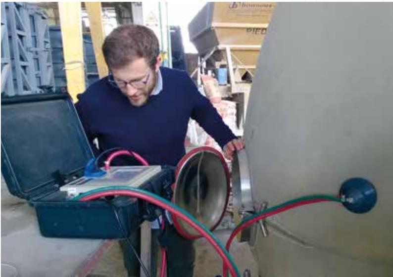
Concrete vessels are increasingly replacing the traditional oak barrels to produce wine. Among other things, micro-oxygenation through the concrete walls seems to help improve the quality of the wine. The technology was first developed in France. Patricio Río running air-permeability tests on the outer and inner surfaces of vessels made in Argentina (to link it to the micro-oxygenation of the wine).
