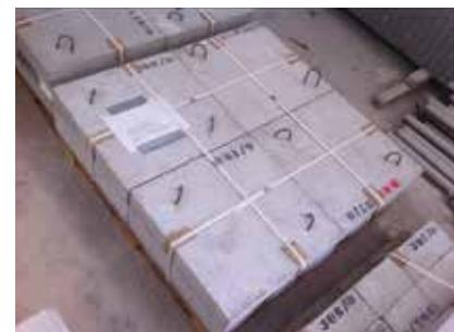
TC 261-CCF (Creep behavior in Cracked Sections of Fiber Reinforced Concrete) Round-Robin Test: pictures of the production process of concrete specimens for the RRT and pallet packaging to deliver all over the world. They produced more than 450 concrete multi-sized specimens in 4 days, which means a considerable production volume. All these specimens were sent to 22 different destinations (Canada, Argentina, Brazil, Japan, India, South Africa, Australia and Europe). Credits: TC 261-CCF
