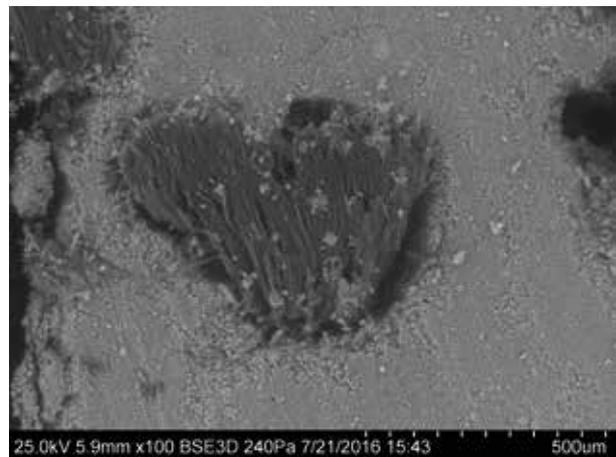
"Hemp concrete" obtained by Scanning Electron Microscope (SEM). The "heart" that appears on the photos represents the wood part (hemp) of the bio-based material. Credits: Kamilia Abahri
