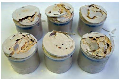
Migné limestone samples containing 1 wt.% of sodium sulfate: resulting damage after re-wetting with pure water. Credits Cristiana Nunes (TC 271-ASC)
