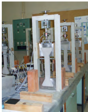
▲ Review of restrained shrinkage tests. Veiga R. et al. RILEM SMSS Convention 2019.
