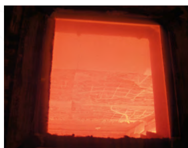
Spalling phenomena observed inside a furnace during a laboratory fire test. Courtesy of Robert McNamee.
