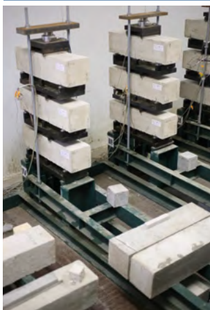
▲ Flexural creep of FRC prismatic specimens. Courtesy of Pedro Serna.
