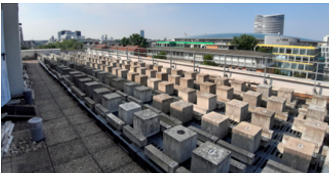
Outdoor exposure site for testing alkali-silica reaction in concrete © VDZ
