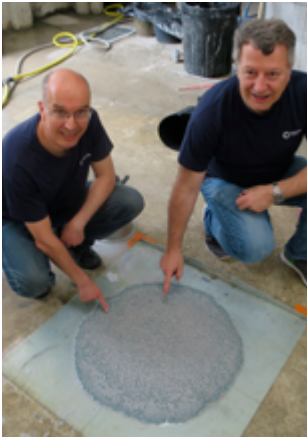
Workability and rheology of SRM 2497 (NIST): Standard Reference Concrete for Rheological Measurements – RRT ©TC 266-MRP
