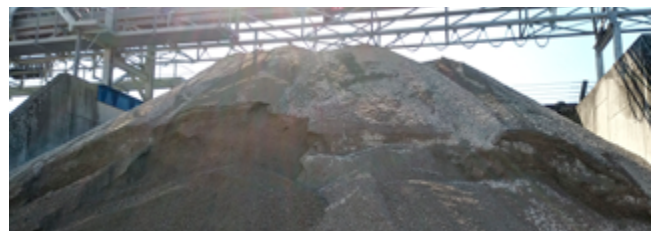
RCA at Concrete Plant ©TC 279-WMR
