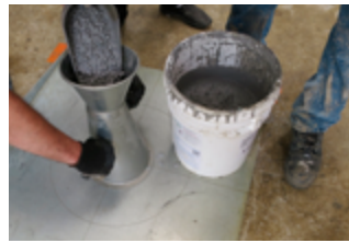
Workability and rheology of SRM 2497 (NIST): Standard Reference Concrete for Rheological Measurements – RRT ©TC 266-MRP
