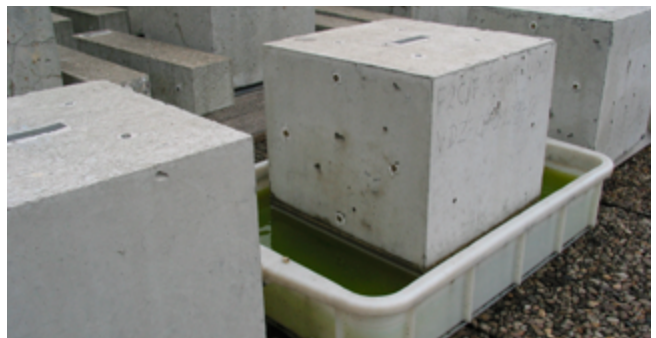
Concrete cubes in outdoor exposure site for testing alkali-silica reaction © VDZ
