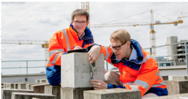
Measuring of outdoor exposed concrete cubes for testing alkali-silica reaction VDZ © Julia Vogel for VDZ
