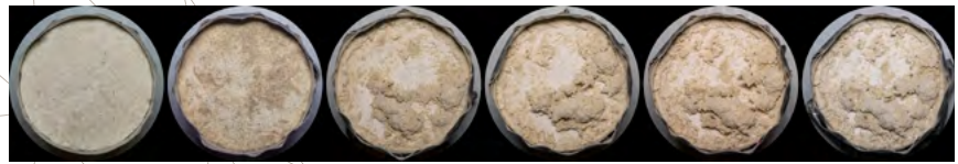
Damage evolution of a Tuffeau specimen upon contamination with 5% sodium sulfate, following the experimental procedure under development by the Technical Committee 271-ASC ©Davide Gulotta, Getty Conservation Institute
