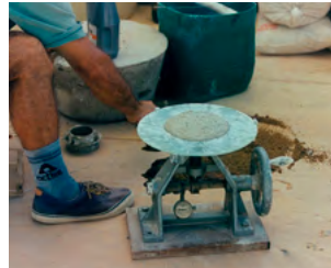
On-site measurements of workability ©Maria Sarantidou, architect
