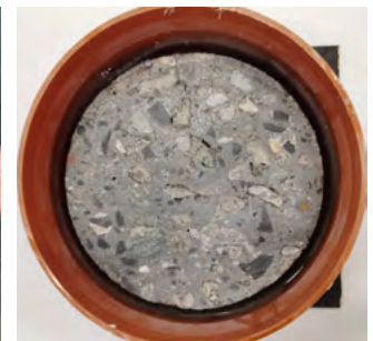
Salt-frost scaling of concrete with 100% Type A+ RCA ©Xiaoguang Chen KU Leuven
