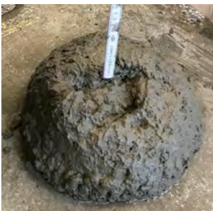
S4 concrete with 100% Type A+ RCA ©Xiaoguang Chen KU Leuven
