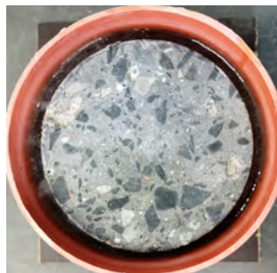
Salt-frost scaling of concrete with 30% Type A+ RCA ©Xiaoguang Chen KU Leuven
