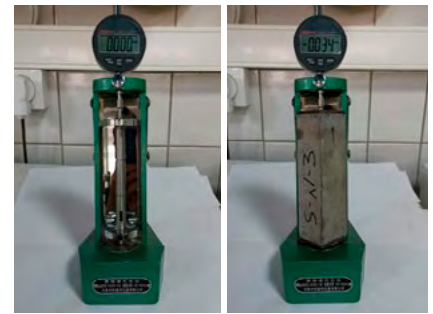
Measurement of the expansion deformations using an electronic indicator mounted on a tripod: a) zeroing the indicator on the reference rod, b) measurement of sample deformations ©V.R. Falikman, TC 286-CEC
