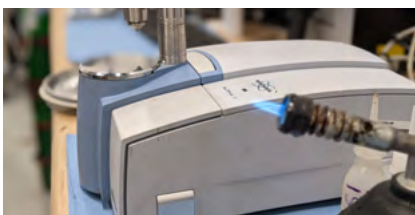
Infrared Spectrometer for Bitumen Analysis in RILEM TC 295-FBB, Task Group 1 ©Dr Johannes Mirwald
