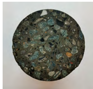
C80-95 concrete with 100% Type A+ RCA ©Xiaoguang Chen KU Leuven
