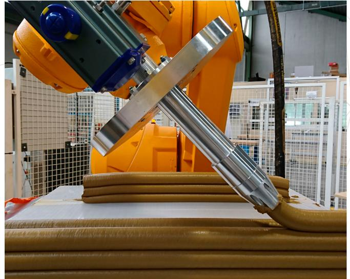
3D printing of earth-based materials. Image courtesy of A. Perrot.
