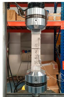
Tensile test on glass FRCM.
