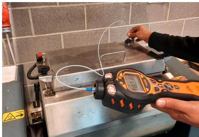
Ion Tiger VOC gas detector using photoionisation (pid). Image courtesy of J. Blom.
