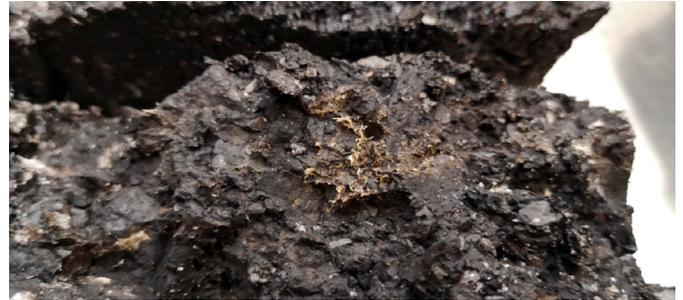
Plastic waste added to asphalt mixture. Image courtesy of Ecole de technologie supérieure, U. du Quebec.
