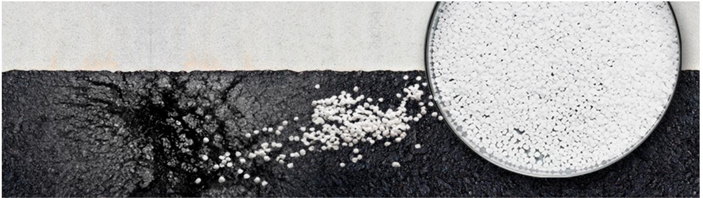
Styrene Butadiene Styrene (SBS) resin. Image courtesy of LG Chem.
