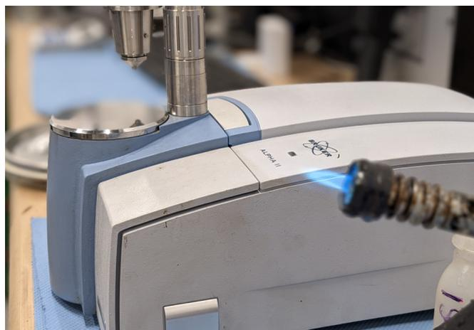
FTIR device to detect chemical composition of bituminous samples. Image courtesy of J. Mirwald.
