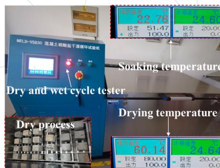
Concrete specimen exposed to solution of sulfate and chloride ions. Image courtesy of Mu Song.
