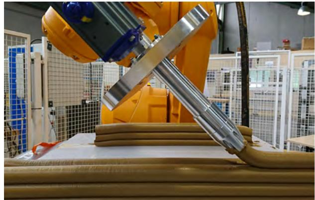
3D printing of earth-based materials. Image courtesy of A. Perrot.
