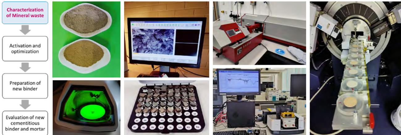
Experimental set-up and processing procedures for characterising and upcycling mineral wastes. Image courtesy of S. Maruthupandian.
