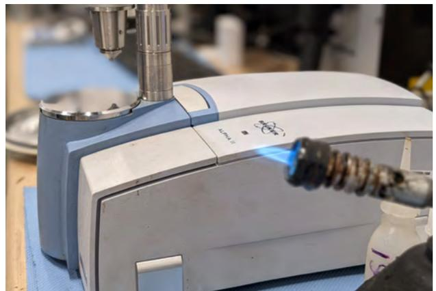
FTIR device to detect chemical composition of bituminous samples. Image courtesy of J. Mirwald.
