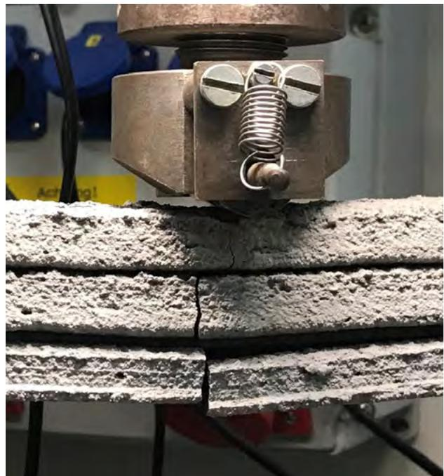
3-point bending testing of a 3D printed concrete specimen. Image courtesy of T. Neef.
