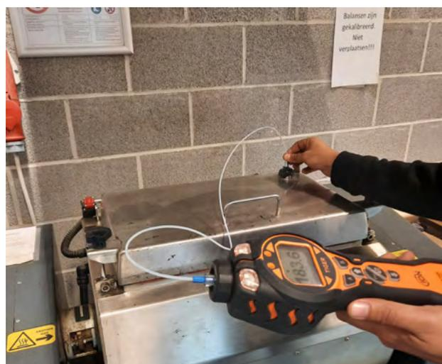
Ion Tiger VOC gas detector using photoionisation (pid). Image courtesy of J. Blom.
