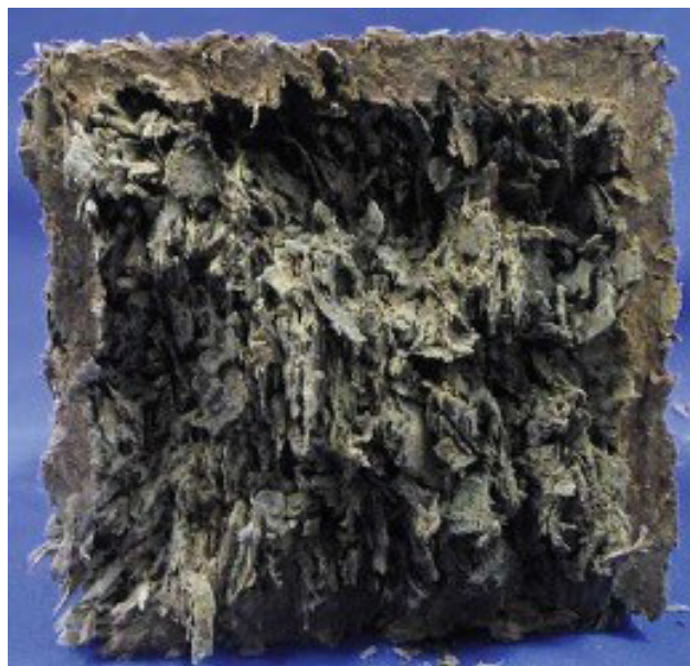
Cross section of wood concrete specimen after shear test. Image courtesy of Yassin Da Gloria.
