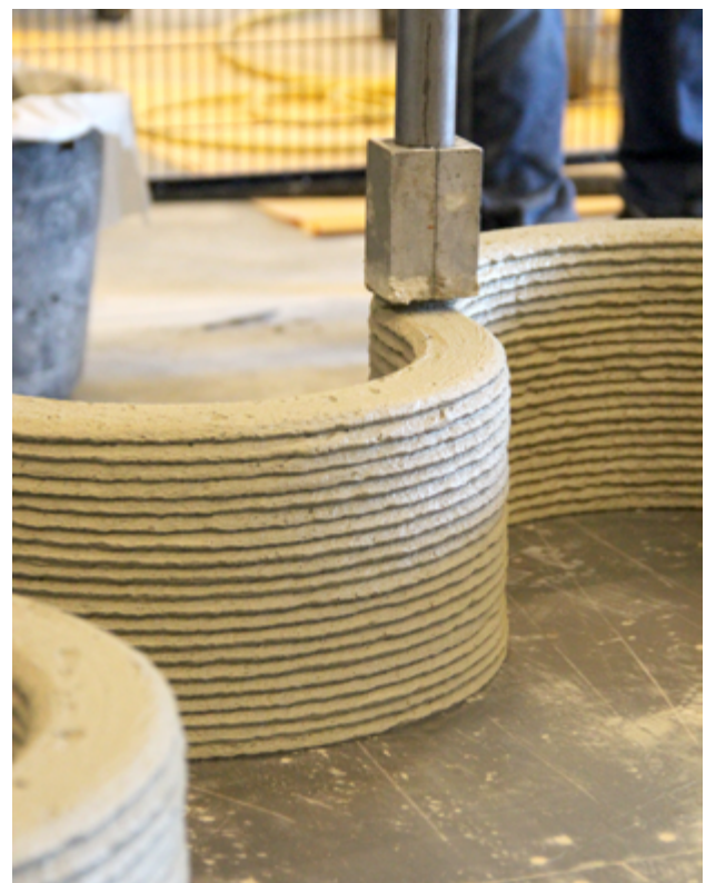
Close up of extrusion-based 3D Concrete Printing process at Eindhoven University of Technology. Image courtesy of Rob Wolf.
