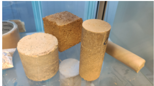
Cast, extruded and compacted earth samples: examples of some of the many processing routes. Image courtesy of A. Perrot.
