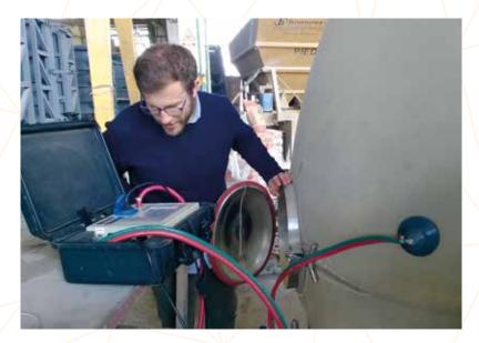
Concrete vessels are increasingly replacing the traditional oak barrels to produce wine. Among other things, micro-oxygenation through the concrete walls seems to help improve the quality of the wine. The technology was first developed in France. Patricio Río running air-permeability tests on the outer and inner surfaces of vessels made in Argentina (to link it to the micro-oxygenation of the wine). Credits: Patricio Río
