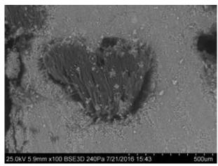
"Hemp concrete" obtained by Scanning Electron Microscope (SEM). The "heart" that appears on the photos represents the wood part (hemp) of the biobased material. Credits: Kamilia Abahri
