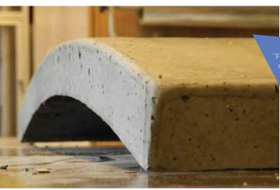
lexible mould" method: a way to manufacture curved concrete elements by deformation after casting; the image shows a demoulded, clearly curved, concrete element of 50 mm thickness.
