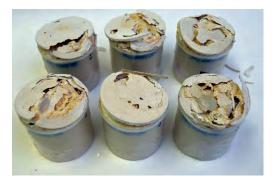
Migné limestone samples containing 1 wt.% of sodium sulfate: resulting damage after re-wetting with pure water.
