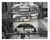
3D DIC monitoring of shell face to track cracks on cement. Pair of high resolution cameras face the middle zone of the TRC shell, where crackings develops. Fine & random black-white speckle pattern covers the TRC face.
