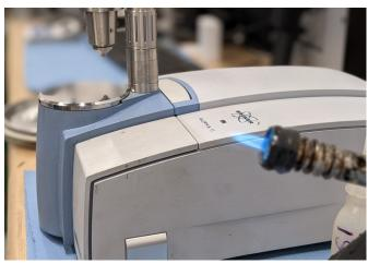
${\sf FTIR}$  device to detect chemical composition of bituminous samples. Image courtesy of J. Mirwald.
