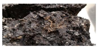
Plastic waste added to asphalt mixture. Image courtesy of Ecole de technologie supérieure, U. du Quebec.
