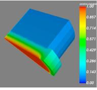
3D - Oxygen concentration map during a diffusion test to illustrate transient effect in sample and in downstream volume as well as side effects because of sealing joints. This work contributes to defining the right analytical solution for interpreting gas diffusion test results. Image courtesy of B. Huet.
