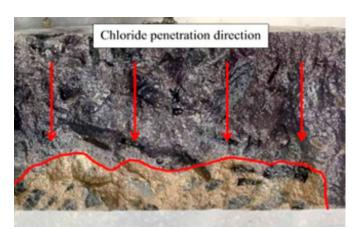
Chloride penetration depth measurement after conducting the chloride migration test NT Build 492. <u>A. Noushini et al. *Materials and Structures* (2021) 54:57.</u>
