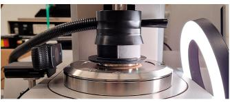
Dynamic Shear Rheometer testing set-up. Image courtesy of O. Baglieri.
