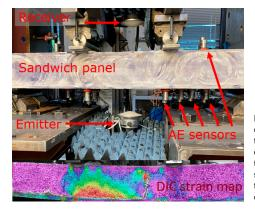
Experimental set up of a 4-point bending test and monitoring equipment to assess the damage of the sample during the test. Image courtesy of D. Angelis.
