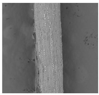
Microscope image of untreated coconut fibre. Image courtesy of O. Kolawole.
