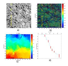
Vegetal aggregate participation: a) picture of hemp concrete of the RRT; b) superposition with vertical strain; c) vertical displacement field; d) section along the yellow line. Image courtesy of É. Toussaint.
