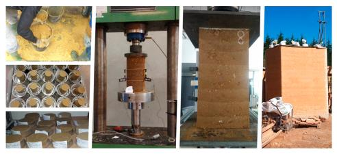
From the left to the middle: preparation and testing of earth-based material samples. On the right: full size (unscaled) rammed earth test wall. Image courtesy of A. Fabbri.
