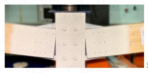
Laboratory testing of a timber joint. Image courtesy of J. Branco.
