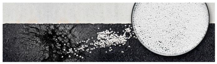
Styrene Butadiene Styrene (SBS) resin. Image courtesy of LG Chem.
