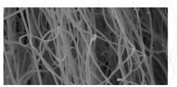
${\sf Electron\ micrograph\ of\ entangled\ Multi-Walled\ Carbon\ Nanotubes.\ Image\ courtesy\ of\ M.\ Liebscher.$
