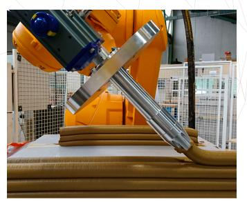
3D printing of earth-based materials. Image courtesy of A. Perrot.
