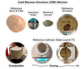
Schematics of preparation and testing of reference cold bitumen emulsion mortars. Image courtesy of A. Graziani.
