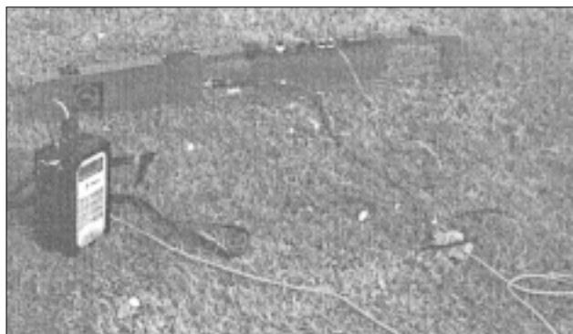
Fig. B.1 – EM 38 Geonics conductivity meter and data logger (by permission of Geonics Limited).
