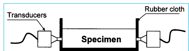
Fig. 5 - Illustration for the UPTT measurement (a side view).
