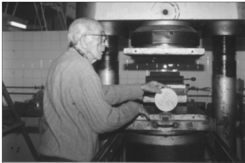
Prof. Carneiro at the Laboratory preparing a cylinder for the Brazilian Test.
