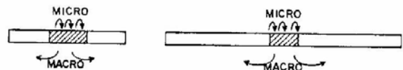
Fig. 5 - Anodic sites S_A present microcell activity in addition to the macrocell formed with the adjacent non-corroding zones, S_C . S_A + S_C = S (total area). Galvanic current may be only a fraction of the total corrosion current.
