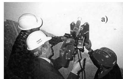
Fig. 1 - Apparatus for adhesion test.
