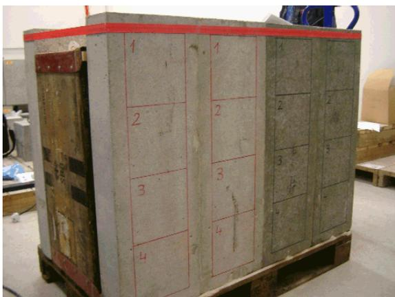
Fig. A2 - Disposition of the slabs for NDT, with the 200 x 200 mm test areas marked.
