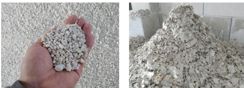
Figure 7: Products of the processing of gypsum plasterboard: Gypsum grains left, cardboard flakes right
