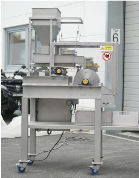
Figure 1: Dry rare-earth separator used in the tests
