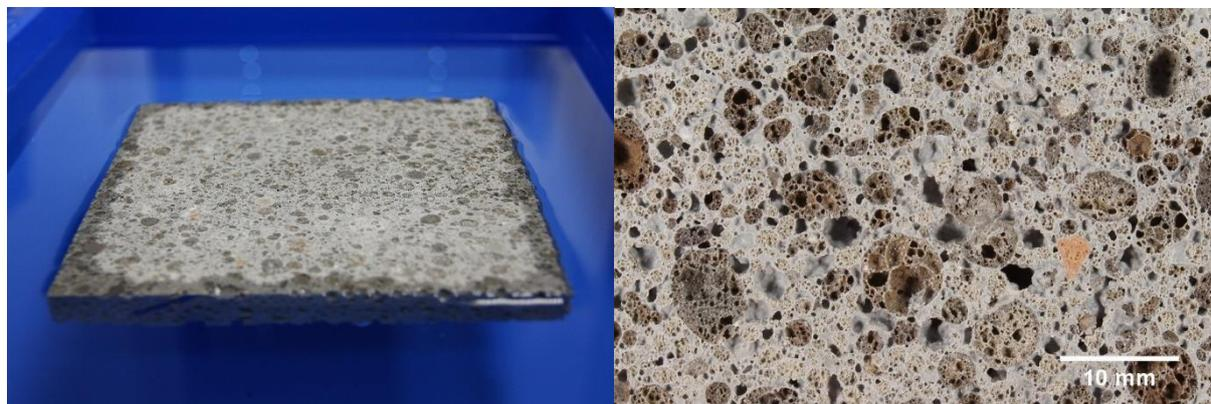
Figure 1: Infra-lightweight concrete floating on water (left), close-up of cut surface area of an infra-lightweight concrete cylinder (right).
