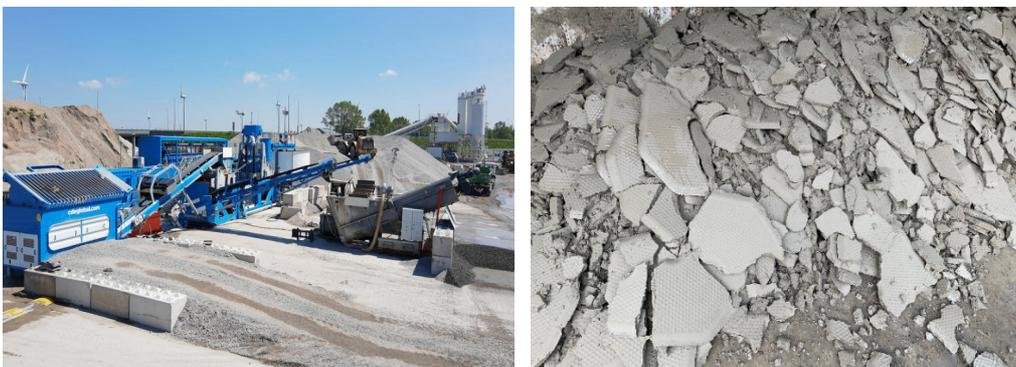
Figure 1: Aggregate washing equipment (left) and washing slurry powder (WSP) (right)
