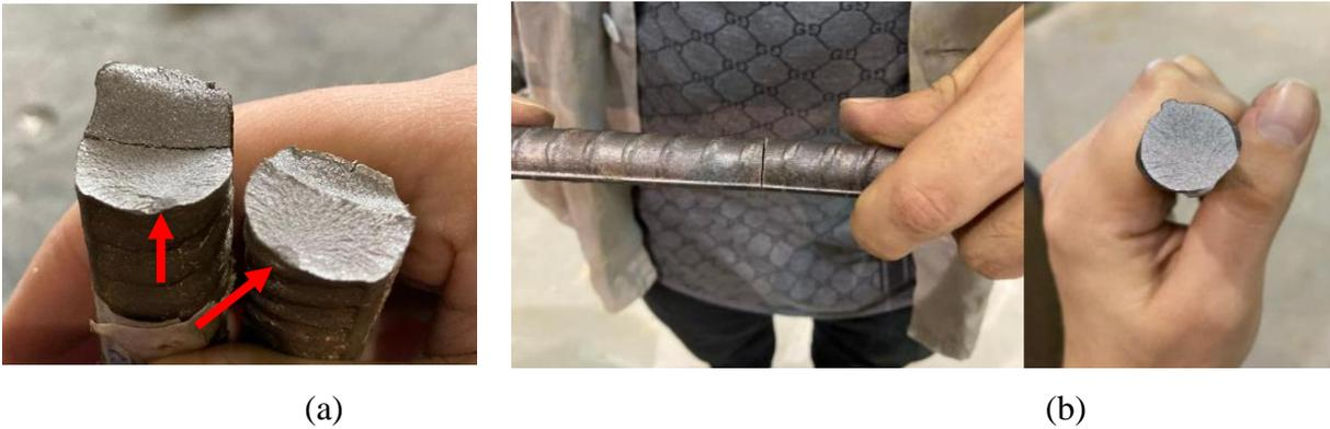
Fig. 4 – Brittle failure of steel rebars (a) rebar collected at the factory building at São Paulo ID3-SP, from an industrial floor, showing signs of fatigue (b) rebar collected from the commercial building at São Bernardo do Campo ID 1 - SBC
