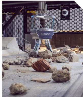
Figure 4: Sensor-based sorting device for the separation of brick and concrete in action in a recycling plant left [3] and heavy picker for sorting construction and demolition waste right [4]
