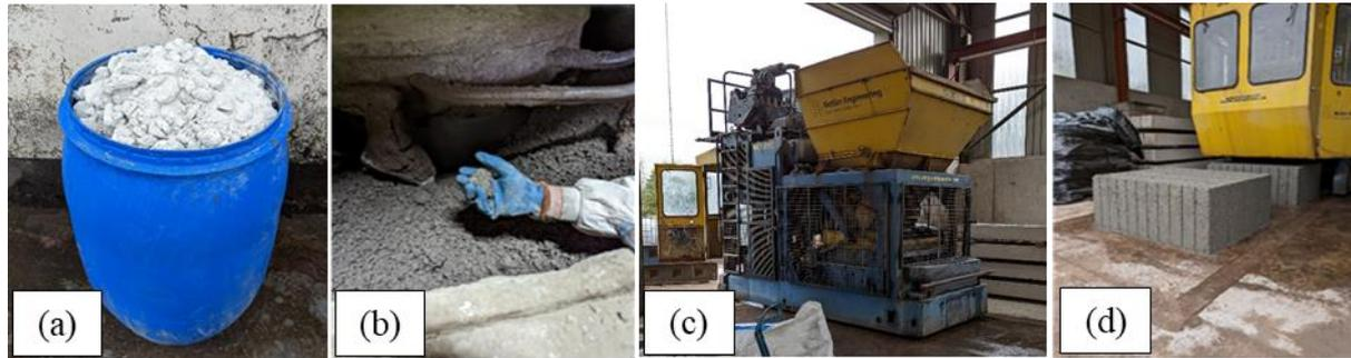
Figure 2: factory trials for the production of alkali activated blocks (a) “clumps” of glass-derived activator (b) squeeze test for workability (c) block making machine (d) cast blocks.
