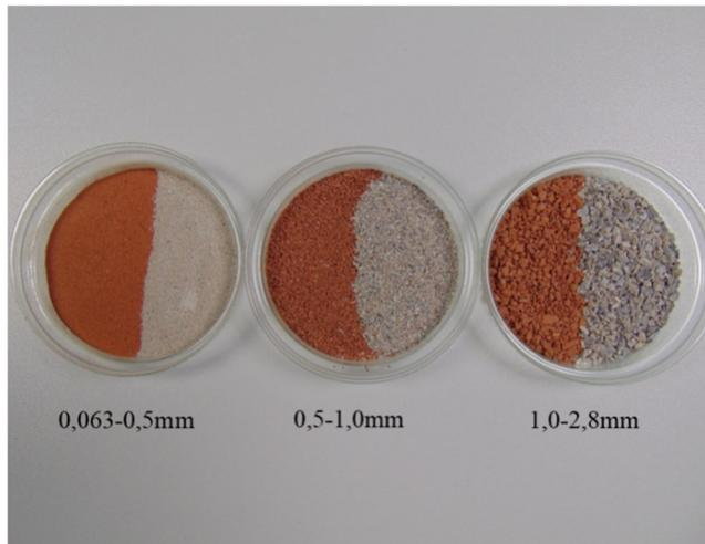
Figure 3: Different fraction of concrete-/brick-mixture before sorting
