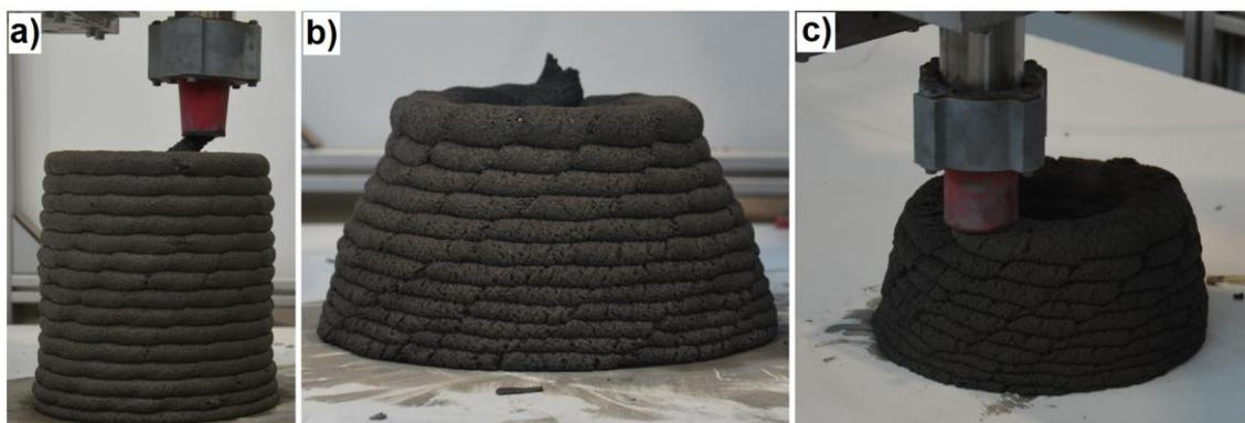
Figure 4: Printing process results: a) specimen R0 during printing; b) specimen R30 after collapse; c) specimen R50 during printing process
