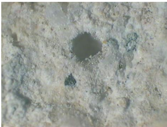
Figure 6a: Secondary crystallization in pores
