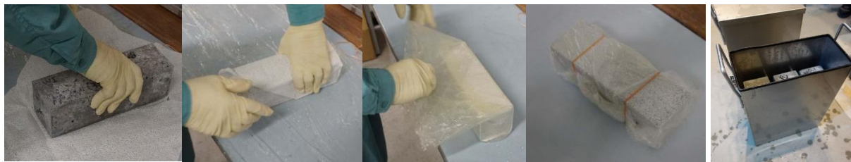
Figure 2: Examples of alkali-wrapping of concrete prisms.
