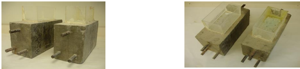
Figure 3. Example of ASTM G109 Test Blocks
