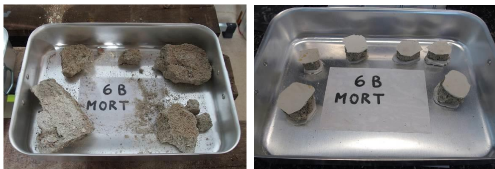
Figure 2: Mortar samples (left) and specimens prepared for testing (right)
