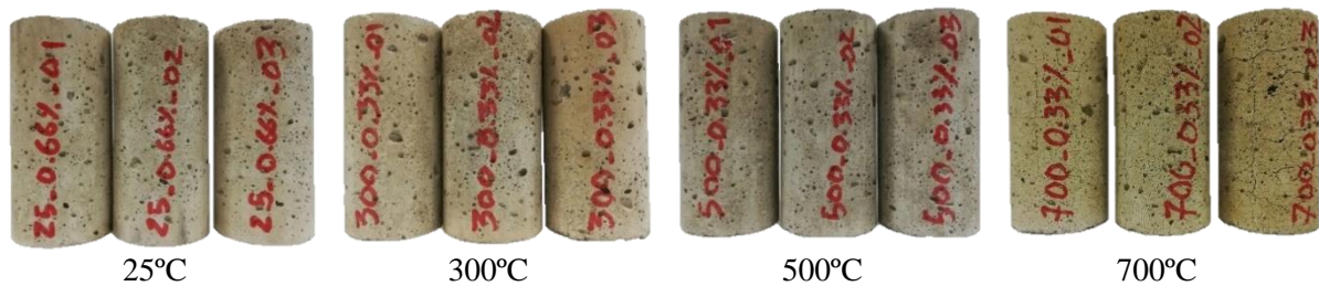
Figure 3: Visual appearance of the specimens after high temperature exposure.
