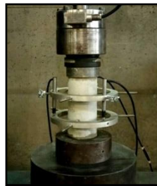
Figure 2: Set-up of static E-modulus
