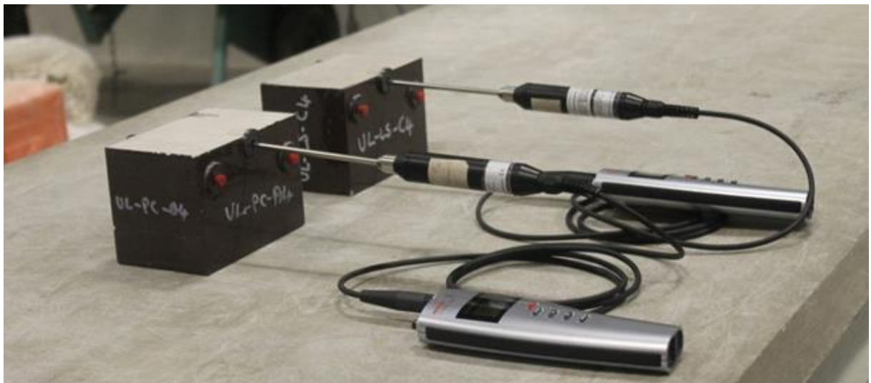
Figure 2: Experimental program for RH measurement
