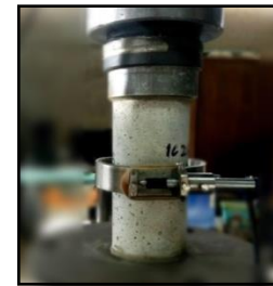
Figure 3: Set-up of Poisson's ratio
