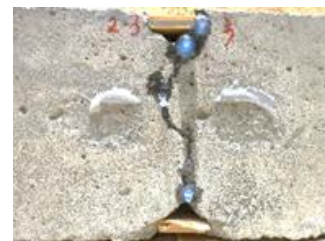
Figure 7: Release of repair agent outside the specimen
