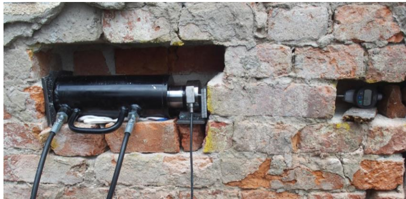
Figure 5: Shear test, building 7 – outside wall
