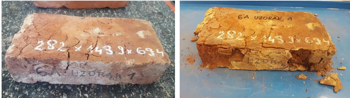
Figure 4: Clay brick specimen before (left) and after testing (right)
