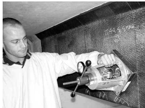
Figure 2: Tensile bond testing of the applied FRP
