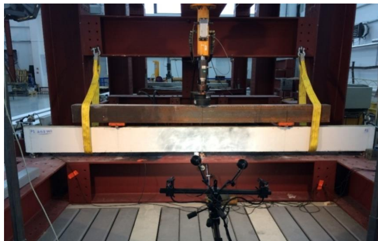
Figure 2: Test setup with beam specimen
