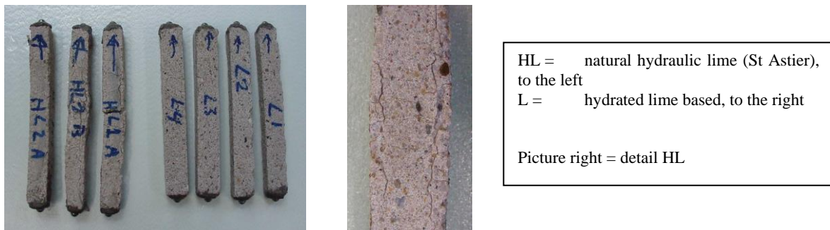
Figure 6: Mortar prisms after 15 weeks in sulfate solution. Natural Hydraulic Lime based (HL) specimens with clear expansion and deformation. Hydrated lime based (L) not any expansion, [10]
