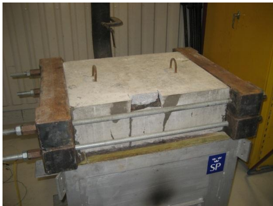
Figure 2: A small slab with externally mounted load arrangement or “cradle”.
