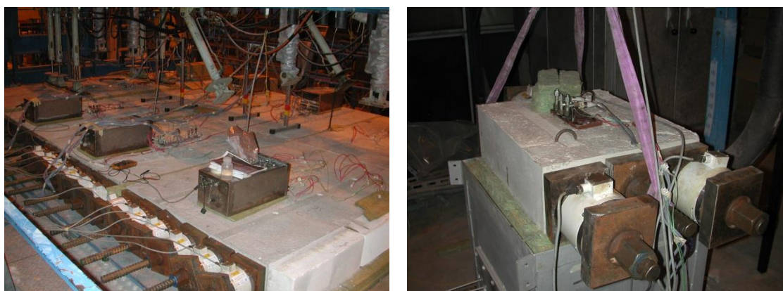
Figure 1: Specimens with internal post-stressing bars. To the left are large slabs and to the right a small slab. Load cells are mounted on the post-stressing bars for load measurements.
