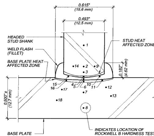
Figure 3: Stud weld cross-section.<sup>1</sup>
