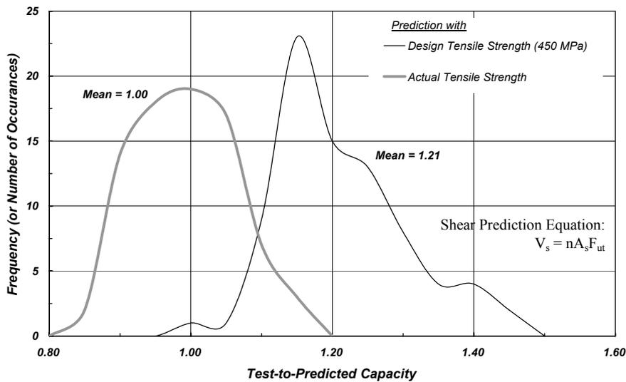
Figure 2: Frequency distribution plot of steel stud failures.
