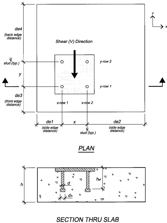
Figure 1: PCI notation for anchorage geometry.<sup>1</sup>
