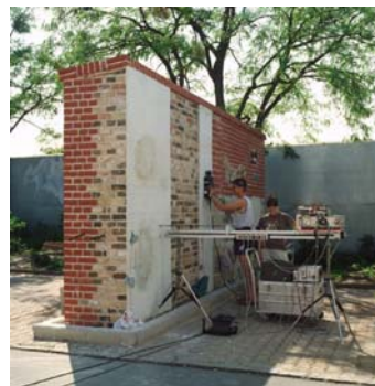
Figure 3a Historic Masonry Specimen “Obelix” at BAM
