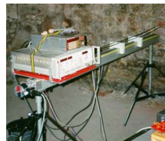
Figure 11 Microwave borehole system for on-site applications
