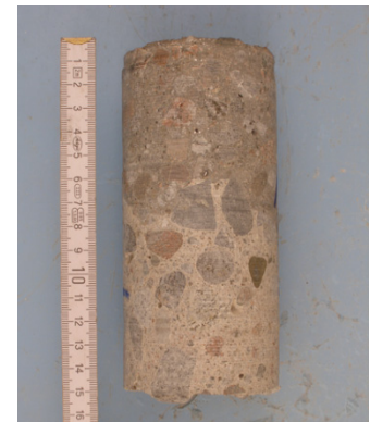
Figure 18: Steel-fibre reinforced concrete overlay
