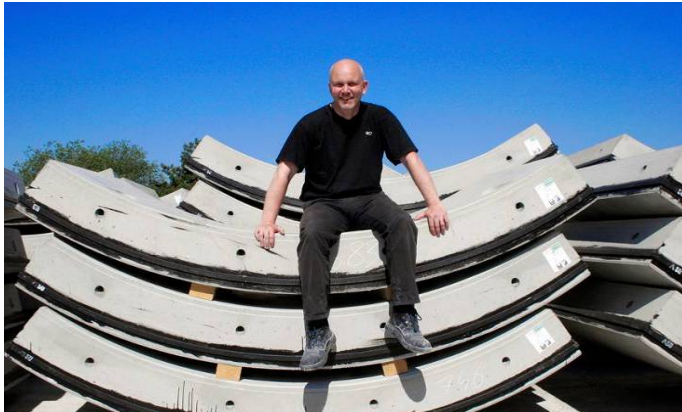
Figure 13: Heating Tunnel Copenhagen with steel-fibre reinforced concrete for the segmental lining
