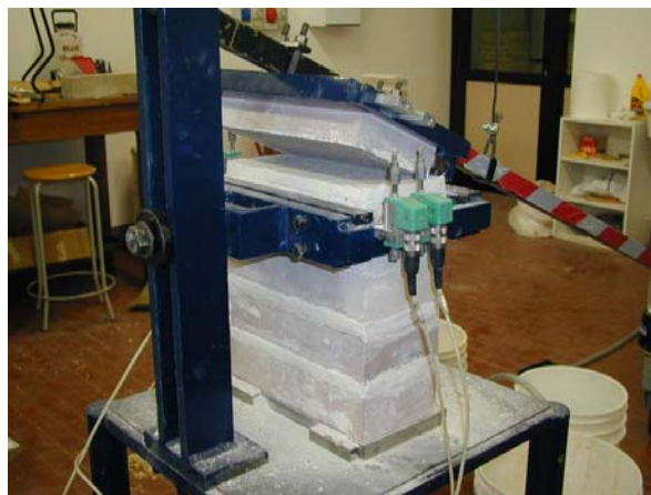
Fig. 4. Loading with water flow (right bottom) and displacement measurement transducers
